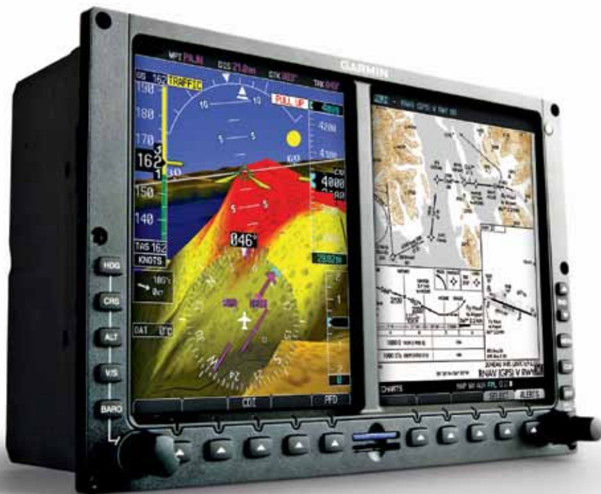
The dual-screen Garmin G600 with synthetic vision technology uses sophisticated graphics modeling to create a 3-D topographic landscape.
