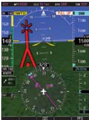
A vertical obstacle, in this case a tower, in red indicating it is in the flight path.
