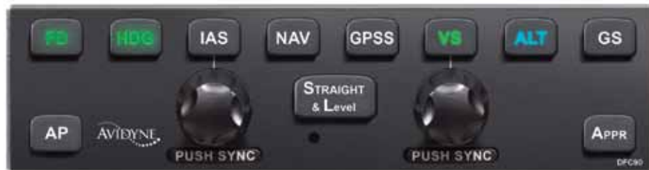
Avidyne's DFC90 autopilot with its envelope protection logic fits in the same panel space as the original unit.
