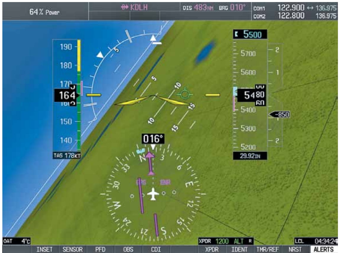
Garmin’s ESP is applying at least 10 pounds of left aileron stick force building to 20 pounds of force in this situation to help the Cirrus pilot recover from the steep bank and nose-low attitude. The double slash marks at the 30-degree bank angle mark shows ESP is active and that 30 degrees is the bank angle recovery target.
