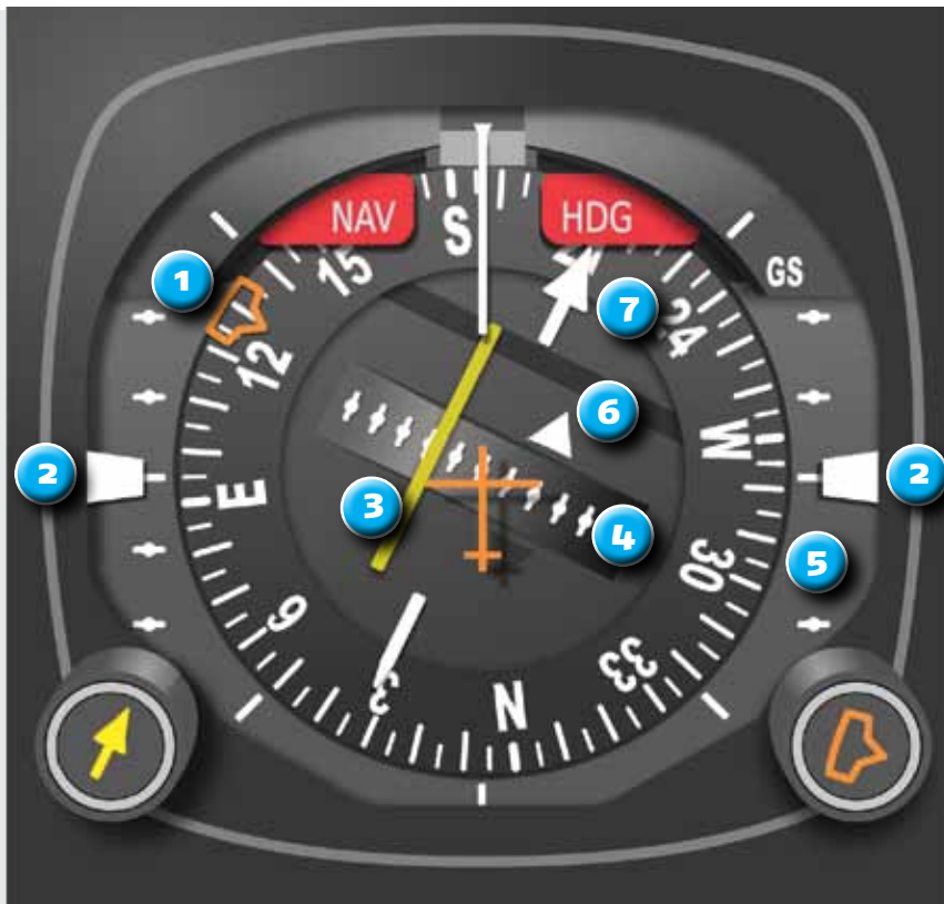
1. Heading Select Bug 2. Glideslope Pointers 3. Course Deviation Bar 4. Course Deviation Scale 5. Glideslope Deviation Scale 6. TO/FROM Indicator 7. Course Select Pointer
